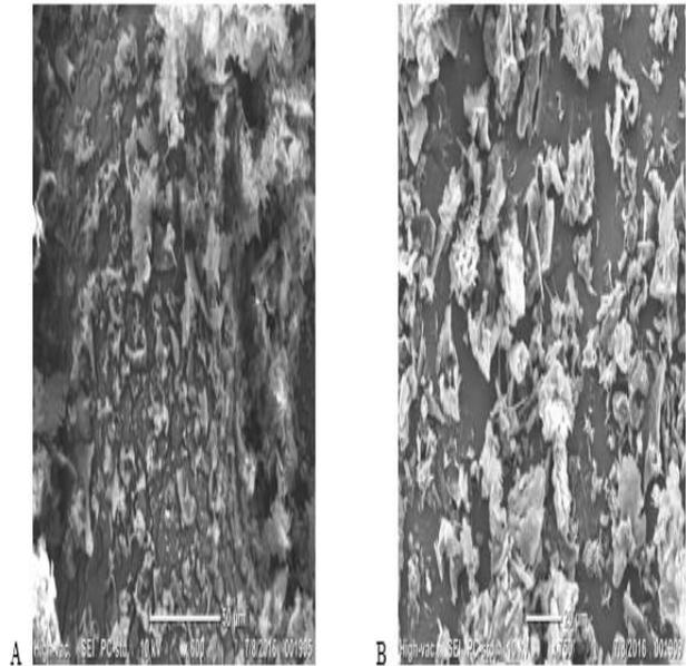
Fig. 5. Scanning electron microscopy of dual matrix beads. A, Unloaded and B, Loaded beads with enzyme
