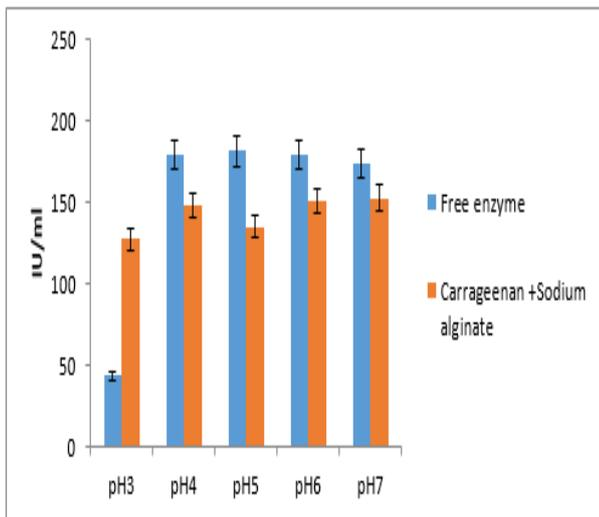
Fig. 4. Comparison of alpha amylase enzyme activity of free enzyme and loaded beads at 50°C.
