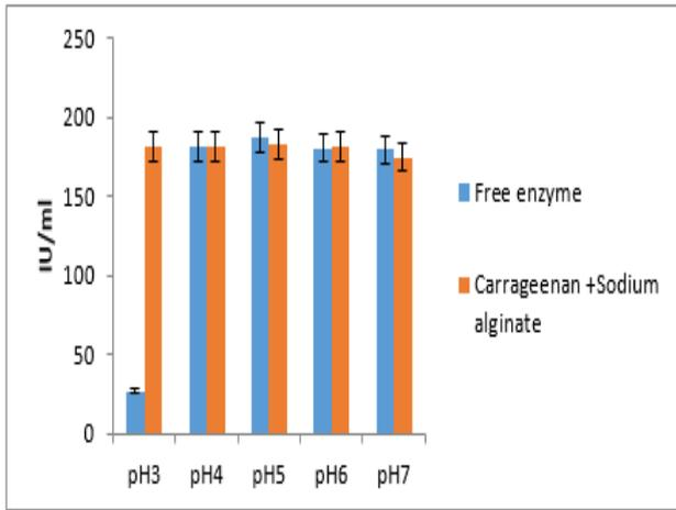
Fig. 3. Comparison of alpha amylase enzyme activity of free enzyme and loaded beads at 37°C.
