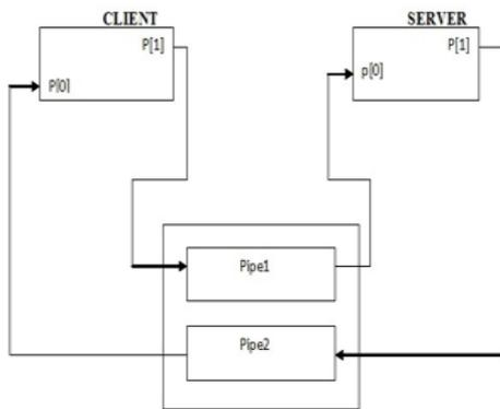
Fig.7. Full Duplex Pipes
