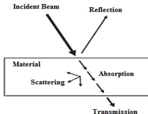
Figure 9. Laser Material Interaction [11]
