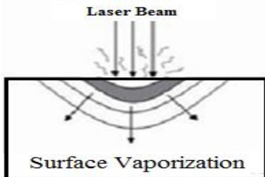
Figure 12. Surface Vaporization Process
