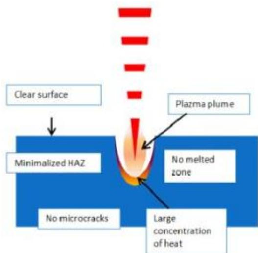
Figure 16(a) Long Pulsed (b) Ultra Short Pulsed Fibre Lasers [13]
