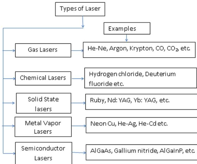
Figure 15. Types of Commonly Used Lasers [13]
