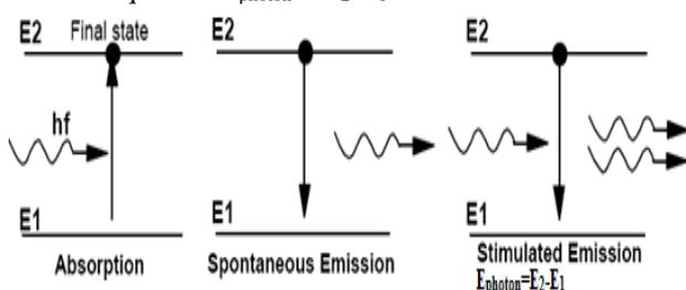
Figure 4: Two Level Energy Level Distribution System (Mishra, 2005) [9]
