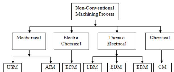
Figure 1. Various Non-Conventional Machining Processes
