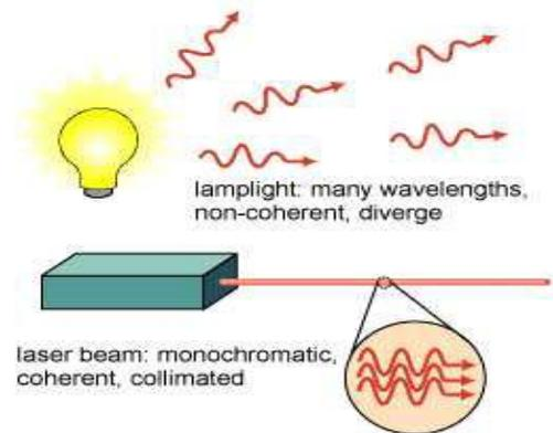
Figure 5: Monochromatic, Coherent and Collimated beam of Radiation [8]
