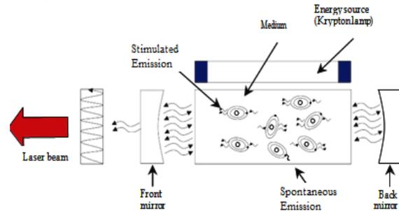
Figure 8. Construction and working Principle of Laser [6]
