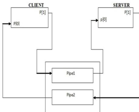
Fig.7. Full Duplex Pipes
