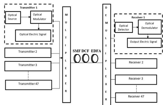
Fig. 1. System setup for 47 DWDM channels at different channel spacing
