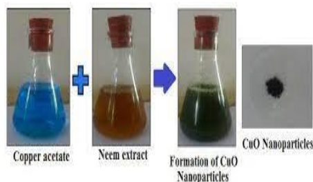
Fig. 2: Synthesis of copper oxide nanoparticles
