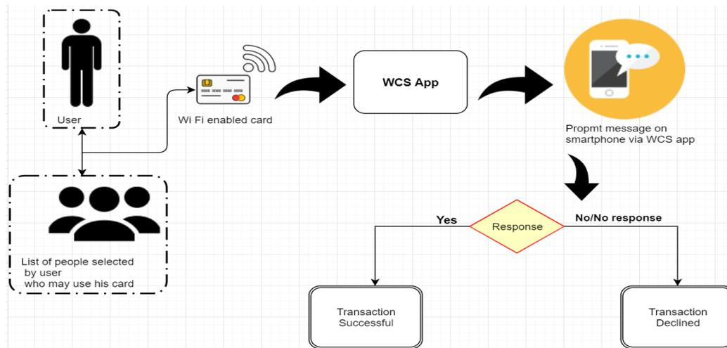
Fig. 3. Working diagram of the proposed system WCS
