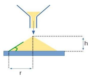
FIG 1: Measurement of an Angle of Repose
