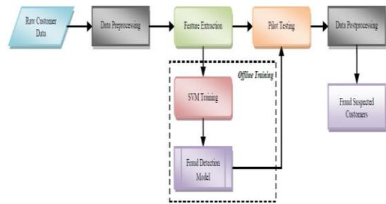
Figure 1: Fraud electricity customer detection framework
